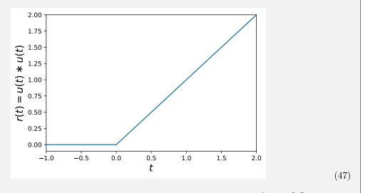
What's the convolution of tu(t) with u(t)? Note that tu(t) = r(t) so this is just  $\int t dt = \frac{1}{2}t^2u(t)$ .
