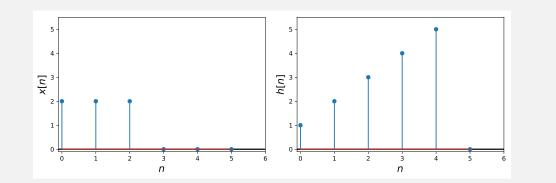
Looking at this graphically, we can see the output is just the superposition of three copies of 2h[k] delayed by 0, 1, and 2, or 2 times sum of three consecutive values of h[k]:
