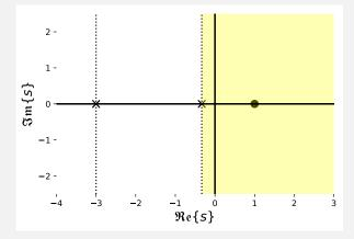
(c) We take the Laplace transform  $\frac{1}{s+1}$  of the input signal and multiply, then do partial fraction
