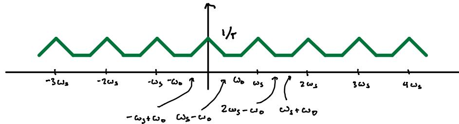
Note that in the first case, we could get back  $X(j\omega)$  (and  $x(t)$ ) by applying a LPF with cutoff  $\omega_0$ :
