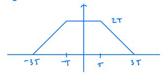
why does this hale rense? The system h acts like a "windowed integrator" - it chops off a 45 length chunch of the supot signal and the convolution integrates that part.
