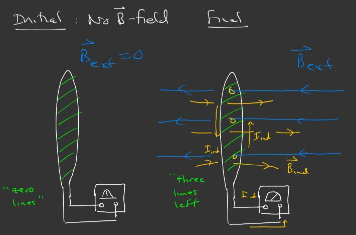
An induced <u>current happens</u> when : The total amount of magnetic field (# of B-field lines) through a loop/coil of wire changes with time. This is called electromagnetic induction.
