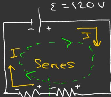
$$R_2 = 144\ \Omega \quad R_1 = 72\ \Omega$$
