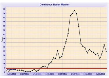
Radon level in this house increased dramatically from one day to the next, because furnace turned on.
